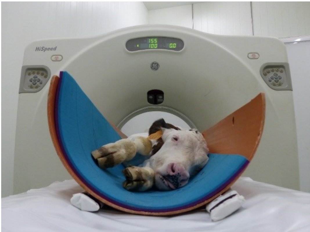
Figure 1: Scanning of a live calf, placed in a polystyrene tube, with computed tomography (CT) equipment
