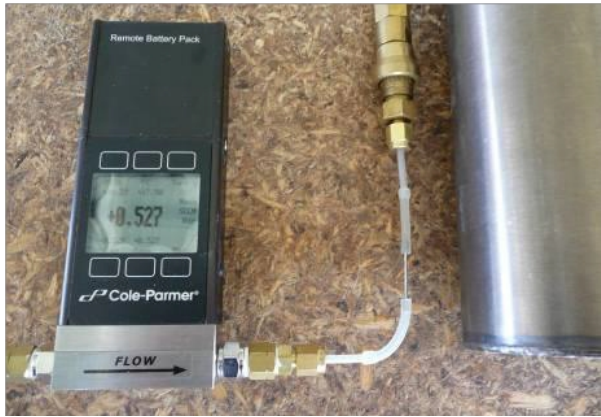
Figure 7: A flow meter on the atmospheric side of the restrictor when measuring flow rate
